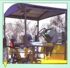
Operator can drive the machine from right-hand side as well as left-hand side as required. The control panel is fitted on sliding base to facilitate this. Thus the operator can work most efficiently and accurately.
